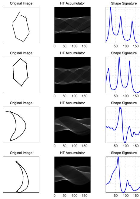
From left to right: image (trajectory), Hough accumulator, shape signature by vertical summation of accumulator
